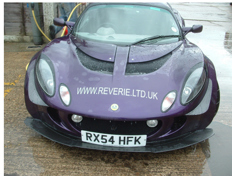
Exige S2 with Front Spoiler & Canards Notice raised centre to accelerate air into Rear diffuser
